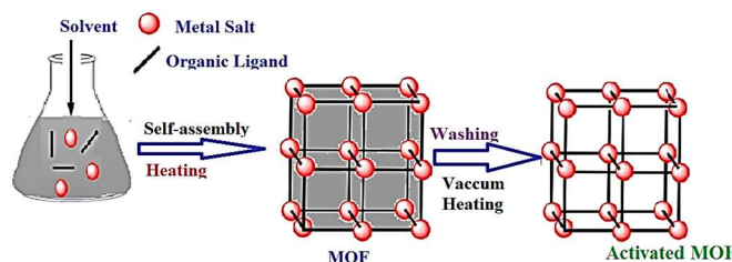
Fig. 2. Typical solvothermal synthesis method.
