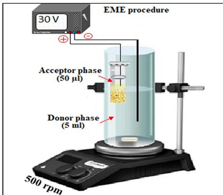
**Fig. 1.** Schematic representation of the proposed EME procedure for the determination of TDF. Extraction conditions: concentration of TDF in water:  $300 \text{ ng ml}^{-1}$ , sample volume: 5.0 ml, acceptor solution volume: 50  $\mu\text{l}$ , applied voltage: 30 V, pH of sample solution: 7.0, pH of acceptor solution: 8.0, extraction time: 15 min, agitation speed: 500 rpm, gel thickness: 4.0 mm, concentration of tragacanth: 2.5% W/V.
