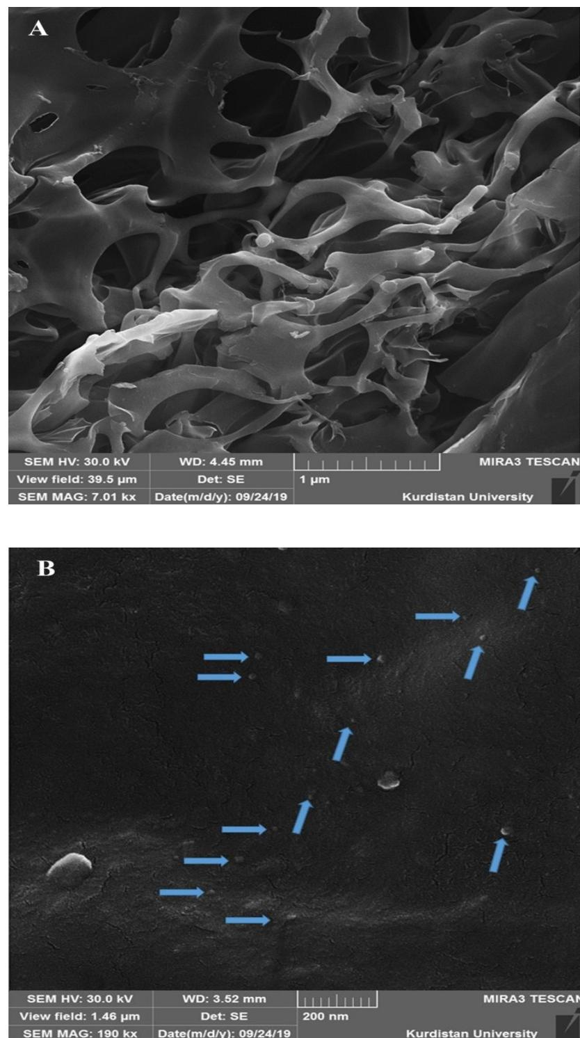
**Fig. 2.** FESEM of AgNPs-tragacanth conjugate gel, (A) the high porosity of the AgNPs tragacanth gel and (B) AgNPs embedded in tragacanth.
