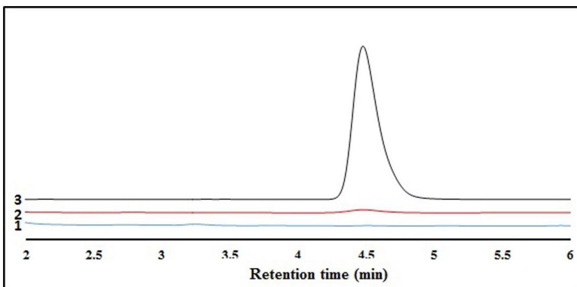
**Fig. 6.** Typical chromatogram for (1) plasma sample, (2) plasma sample spiked with 300 ng ml<sup>-1</sup> of TDF before extraction and (3) plasma sample spiked with 300 ng ml<sup>-1</sup> of TDF after extraction.
