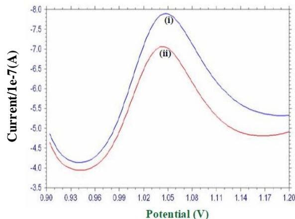
**Fig. 6.** Differential pulse voltammograms of (i) SDN and (ii) SDN in presence of 1mM citric acid.
