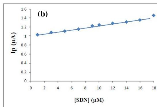
**Fig. 5.** (a) Square wave voltammograms of SDN at different concentrations at (i) 1, (ii) 3, (iii) 5, (iv) 7, (v) 9, (vi) 10, (vii) 12  $\mu\text{M}$ , (viii) 14, (xi) 16 and (x) 18  $\mu\text{M}$ . (b) Plot of the peak current against concentration of SDN.
