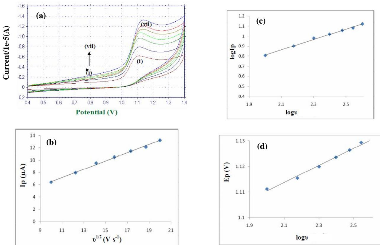
**Fig. 3.** (a) Cyclic voltammograms obtained for 1.0 mM SDN in buffer solution of pH 3.0 at scan rates of (i) 100, (ii) 150, (iii) 200, (iv) 250, (v) 300, (vi) 350 and (vii) 400  $\text{mV s}^{-1}$ . (b). Linear relationship between the peak currents and the square root of scan rate. (c). Linear relationship between the logarithmic peak currents and the logarithmic scan rates. (d). Variation of peak potential with  $\log v$  for 1.0 mM SDN.
