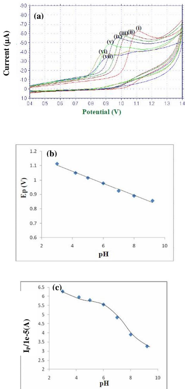
**Fig. 2.** (a) Cyclic voltammograms obtained for 1.0 mM SDN in buffer solution at (i) pH 3.0, (ii) pH 4.2, (iii) pH 5.0, (iv) pH 6.0, (v) pH 7.0, (vi) pH 8.0 and (vii) pH 9.2 with potential scan rate  $100 \text{ mV s}^{-1}$ . (b) Variation of peak potential with pH for 1.0 mM SDN. (c) Variation of peak current with pH for 1.0 mM SDN.
