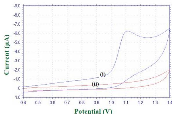
**Fig. 1.** Cyclic voltammograms obtained for 1.0 mM sulfadoxine (SDN) on GCE in pH 3.0, 0.2 M buffer: (i) GCE with SDN (ii) GCE without SDN at scan rate 100 mV s<sup>-1</sup>.
