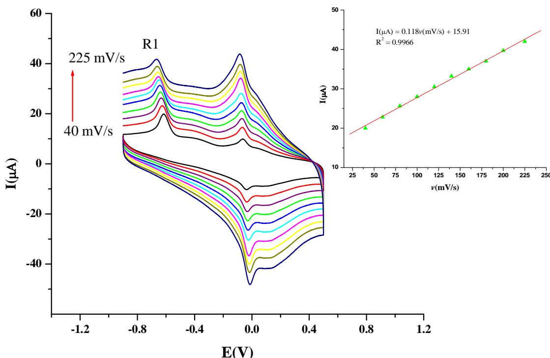
**Fig. 6.** The cyclic voltammograms of 40  $\mu\text{M}$  fenitrothion in 0.1 M phosphate buffer solution (pH 6.0) on MWCNT/GCE at various scan rates (40, 60, 80, 100, 120, 140, 160, 180, 200 and 225  $\text{mV s}^{-1}$ ). Inset: plot of reduction peak current vs. scan rate.
