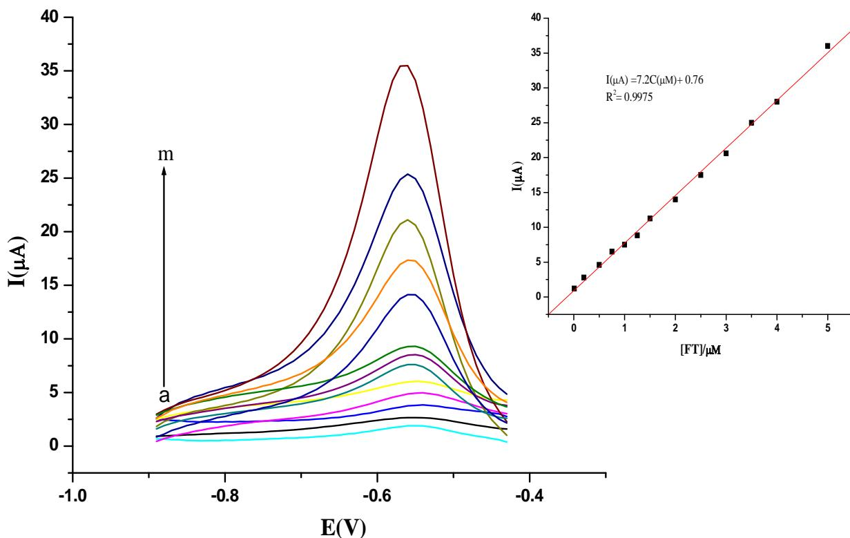
**Fig. 8.** Square wave voltammograms of various concentrations of fenitrothion (a) 0.01  $\mu\text{M}$ , (b) 0.2  $\mu\text{M}$ , (c) 0.5  $\mu\text{M}$ , (d) 0.75  $\mu\text{M}$ , (e) 1.0  $\mu\text{M}$ , (f) 1.25  $\mu\text{M}$ , (g) 1.5  $\mu\text{M}$ , (h) 2.0  $\mu\text{M}$ , (i) 2.5  $\mu\text{M}$ , (j) 3.0  $\mu\text{M}$ , (k) 3.5  $\mu\text{M}$ , (l) 4.0  $\mu\text{M}$  and (m) 5.0  $\mu\text{M}$ .
