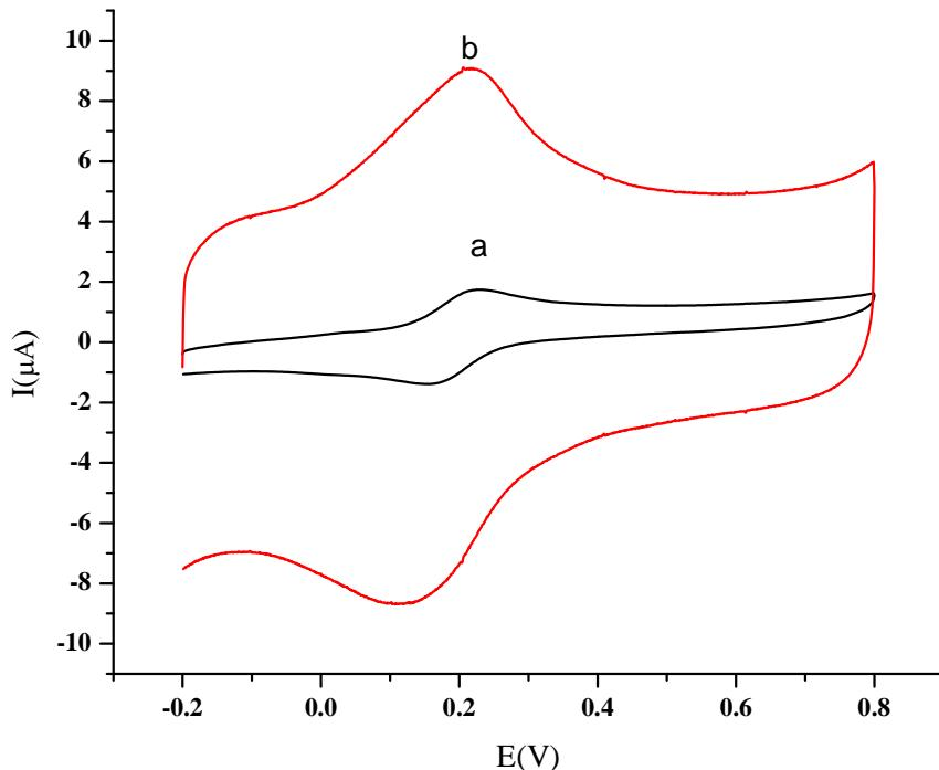
**Fig. 2.** Cyclic voltammograms of 0.1 mM  $\text{Fe}(\text{CN})_6^{4-}$  in 0.1 M KCl on (a) GCE and (b) MWCNT/GCE at a scan rate of  $100 \text{ mV s}^{-1}$ .
