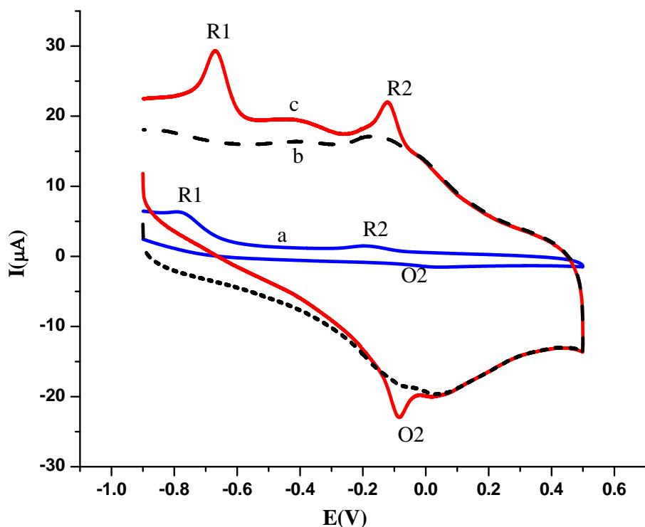
**Fig. 3.** Cyclic voltammograms of 40  $\mu$ M fenitrothion solutions at GCE in 0.1 M PBS pH 7 (a), 0.1 M phosphate buffer solution (pH 7.0) at MWCNT/GCE (b) and 40  $\mu$ M fenitrothion solution in 0.1 M PBS pH 7 at MWCNT/GCE(c). Scan rate: 100 mV s<sup>-1</sup>.
