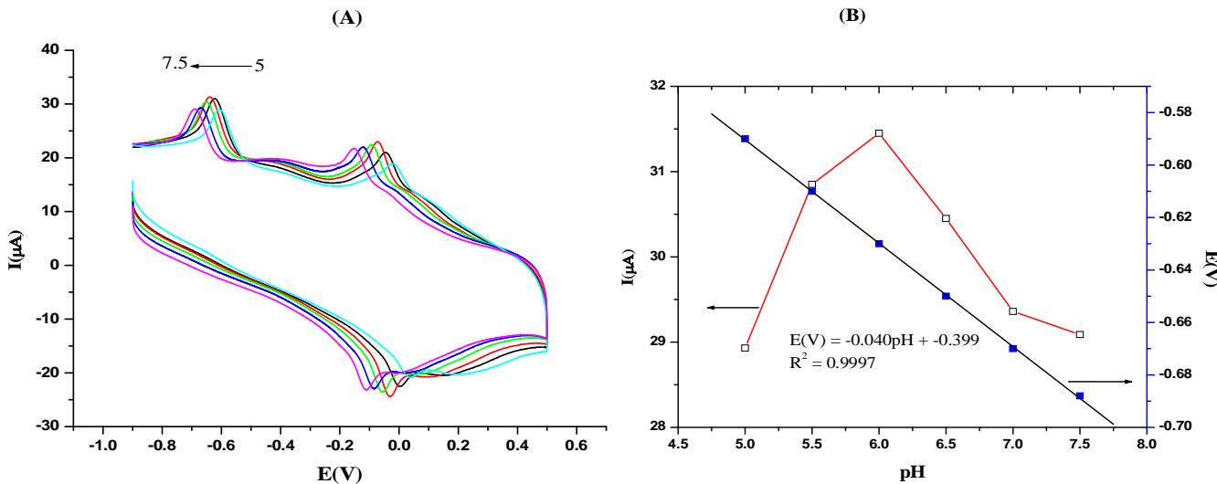
**Fig. 5.** (A) Cyclic voltammograms of 40  $\mu\text{M}$  fenitrothion in 0.1 M phosphate buffer solution at various pH values
