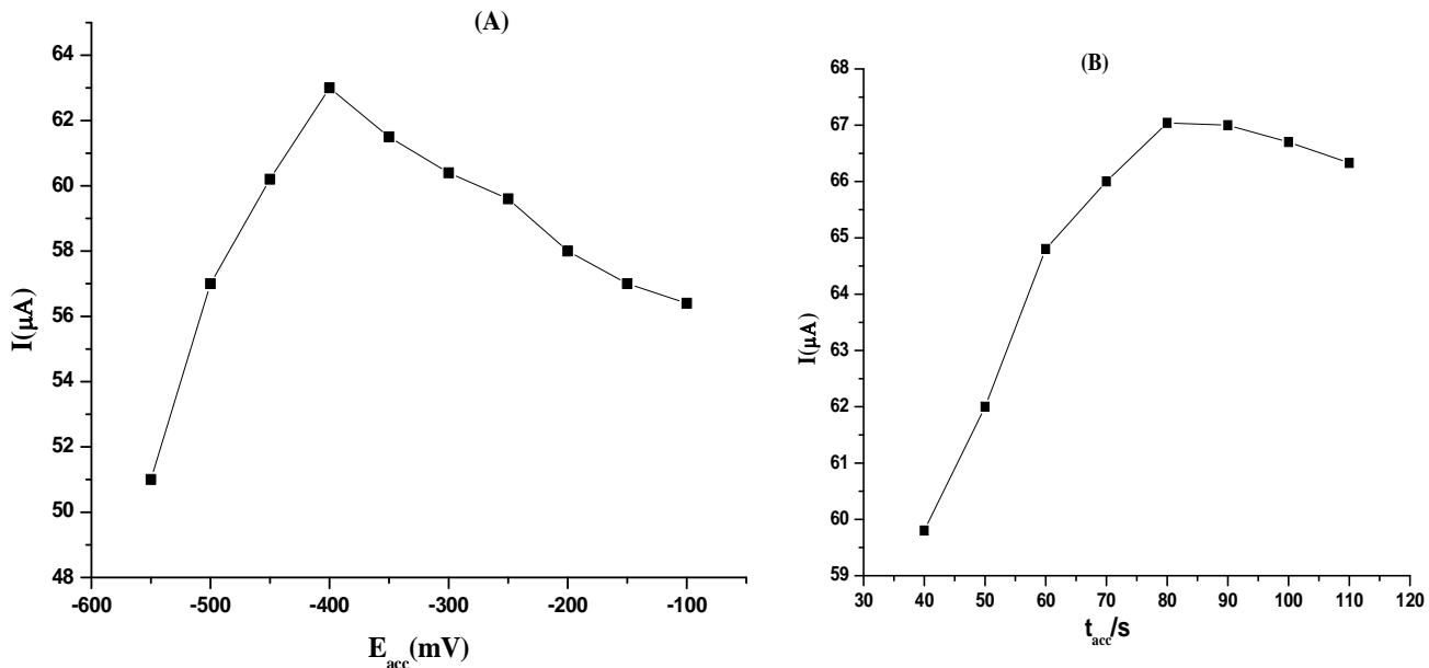
**Fig. 7.** Effects of (A) accumulation potential and (B) accumulation time on peak current of 40  $\mu\text{M}$  fenitrothion in 0.1 mM phosphate buffer solution of pH 6.0 at MWCNT/GCE.
