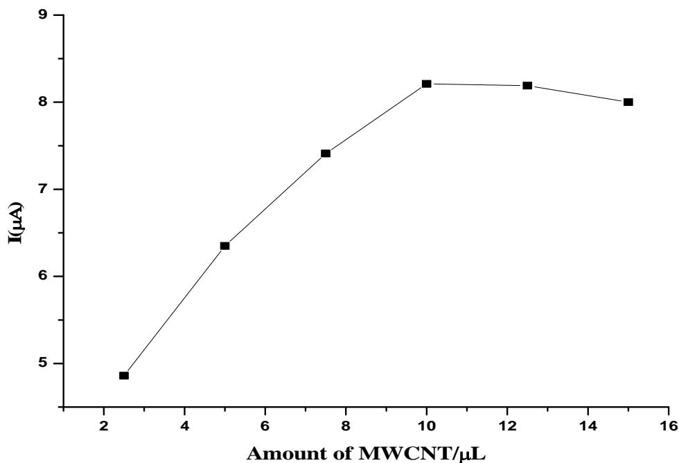
**Fig. 4.** Effect of MWCNTs on reduction peak current of 40  $\mu\text{M}$  fenitrothion in 0.1 M phosphate buffer solution (pH 7.0) at 100  $\text{mV s}^{-1}$ .
