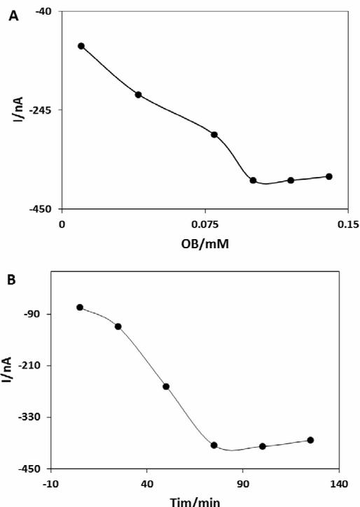
**Fig. 4.** Optimization of the (A) Oracet blue concentration and (B) time span.
