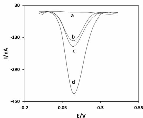
**Fig. 5.** DPV voltammograms of the Oracet blue accumulated on the hybridized oligonucleotides with the immobilized thiolated probes on the electrode, representing the selectivity of the biosensor.
