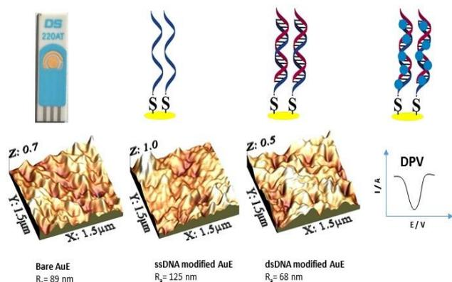
**Scheme 1.** A schematics of the electrochemical biosensor developed for the detection of bacterial DNA and AFM imaging of the working electrode in each modification steps
