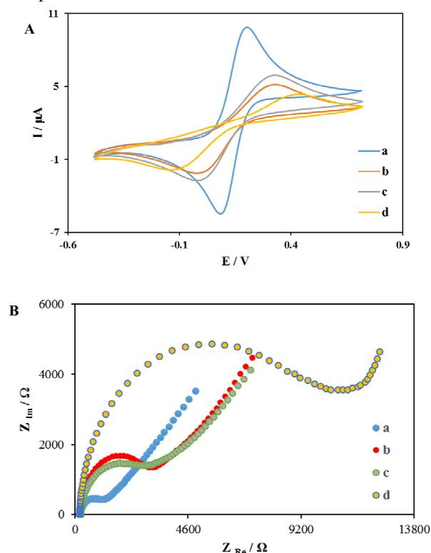
**Fig 1.** Biosensor fabrication assessment, using (A) Cyclic Voltammetry (CV) in 1.0 mM  $[\text{Fe}(\text{CN})_6]^{3-/4-}$  and (B) electrochemical impedance spectroscopy (EIS) in 5.0 mM  $[\text{Fe}(\text{CN})_6]^{3-/4-}$ . In both CV and EIS studies, curve (a) is for bare gold electrode, (b) is ssDNA modified, (c) MCH-ssDNA modified and (d) dsDNA modified gold electrode.
