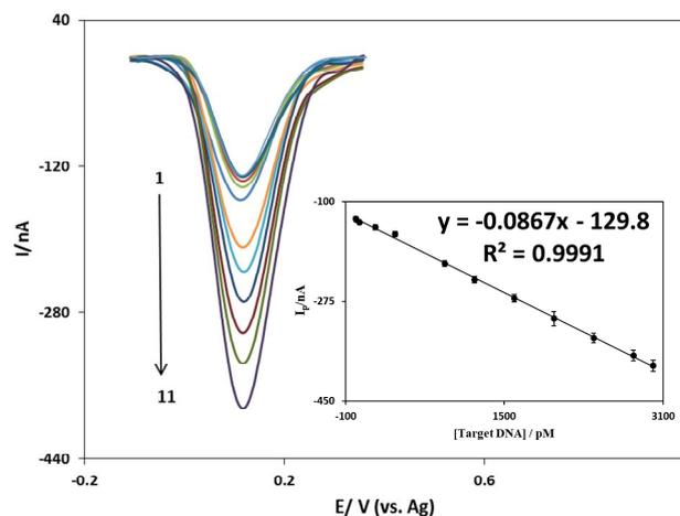
**Fig. 6.** DPV voltammograms of the Oracet blue accumulated on the different concentrations of the target DNA hybridized with immobilized probe on the electrode surface. Inset shows the plot of reduction peak currents of the Oracet blue versus the concentration of the target DNA as the calibration curve.
