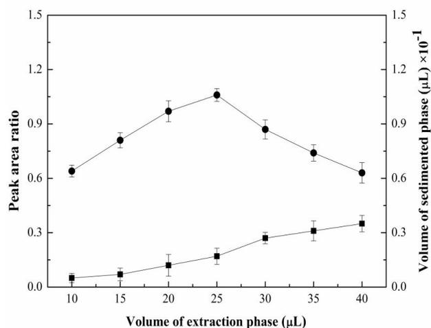
**Fig. 2.** Effect of the extraction solvent volume on the peak area ratio of 2-phenylethanol and relationship between initial extraction solvent volume and sedimented phase volume. Extraction conditions: volume of the disperser solvent (ethanol), 0.6 ml; concentration of NaCl, (0% w/v); pH, 7.0; extraction time, 1 min.
