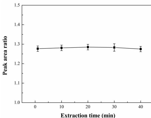
**Fig. 4.** Effect of the extraction time on the peak area ratio of 2-phenylethanol. Extraction conditions: volume of the disperser solvent (ethanol), 0.6 ml; volume of the extraction solvent (CCl<sub>4</sub>), 25  $\mu$ l; concentration of NaCl, (4% w/v); pH, 6.0.
