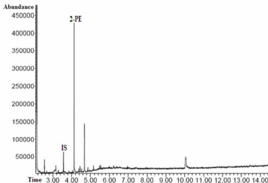
**Fig. 5.** Total ion chromatogram of unspiked rose water sample after DLLME obtained under optimized conditions.
