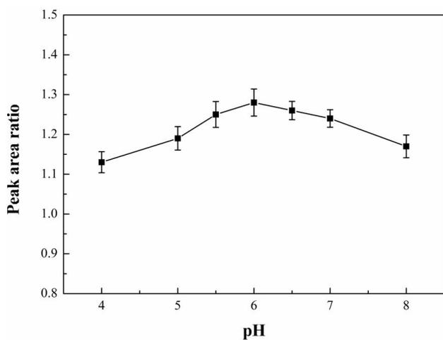
**Fig. 3.** Effect of pH on the peak area ratio of 2-phenylethanol. Extraction conditions: volume of the disperser solvent (ethanol), 0.6 ml; volume of the extraction solvent (CCl<sub>4</sub>), 25  $\mu$ l; concentration of NaCl, (4% w/v); extraction time, 1 min.
