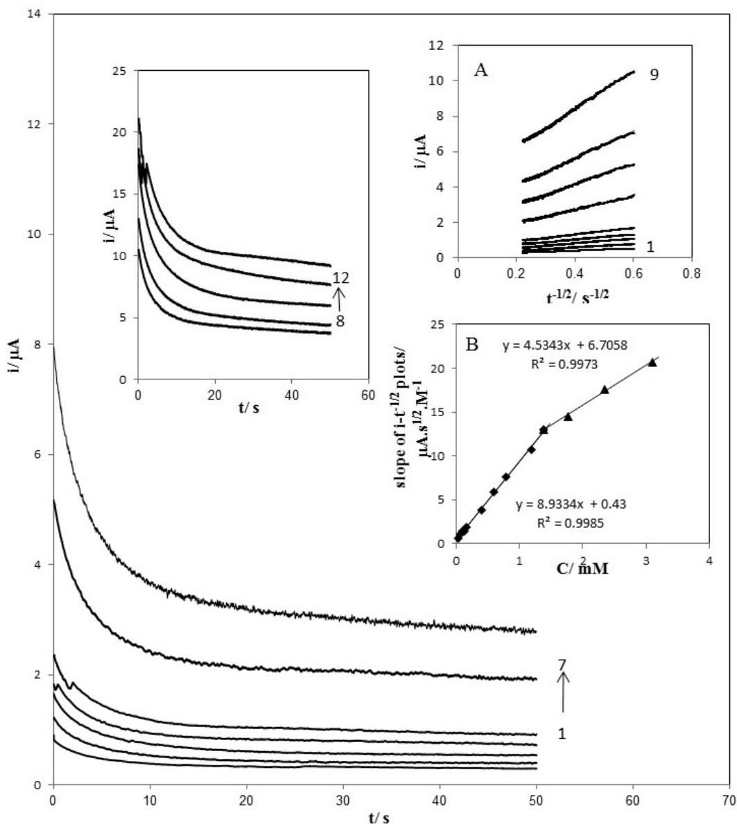
**Fig. 4.** Chronoamperometric response of a poly (EBT)/GCE in 0.1 M ammonium buffer solution (pH 9) containing different concentrations of INH for a potential step of 400 mV vs. SCE. The numbers 1-12 correspond to  $2.90 \times 10^{-5}$ - $3.10 \times 10^{-3}$  M of INH. Insets: Plots of  $I_p$  vs.  $t^{-1/2}$  (A) and the relationship between the slope of the linear segments vs. the INH concentration (B).
