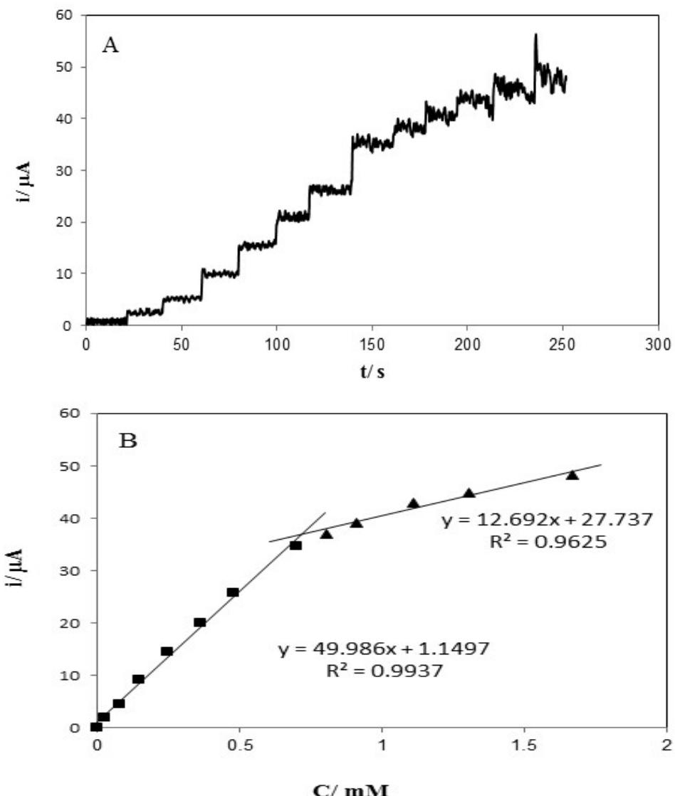
**Fig. 7.** A) Amperometric response of a poly (EBT) modified glassy carbon electrode kept in 400 mV in 0.1 M ammonium buffer solution pH 9 containing different concentrations of INH from  $2.90 \times 10^{-5}$  to  $1.67 \times 10^{-3}$  M. B) Calibration plot of INH.
