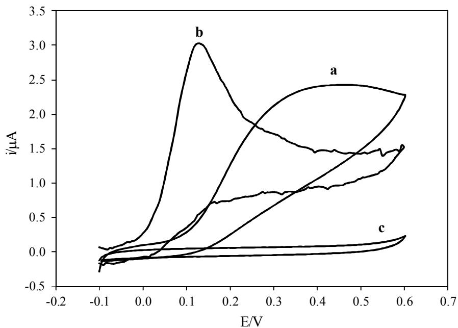
**Fig. 1.** Cyclic voltammograms of 0.25 mM INH at a bare (a) and modified (b) glassy carbon electrode in pH 9  $\text{NH}_3/\text{NH}_4\text{Cl}$  buffer solution. The voltammogram of (c) is the background.
