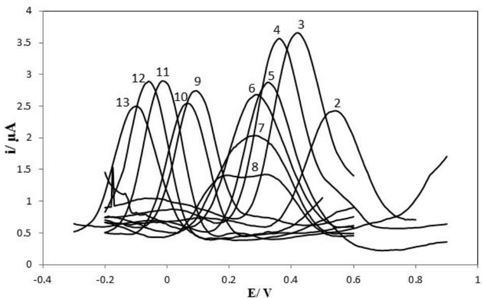
**Fig. 2.** Differential pulse voltammograms recorded for a 1 mM concentration solution of INH at scan rate of  $50 \text{ mV s}^{-1}$  in 0.04 M Britton-Robinson buffer at various pH values from 2 to 13.
