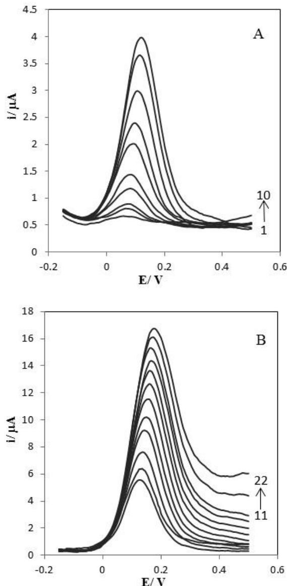
**Fig. 5.** Differential pulse voltammograms for increasing concentrations of INH from (1)  $8.0 \times 10^{-6}$  to (21)  $1.18 \times 10^{-3}$  M in buffer solution (pH 9.0) on poly (EBT)/GC electrode. Scan rate was  $50 \text{ mV s}^{-1}$ .
