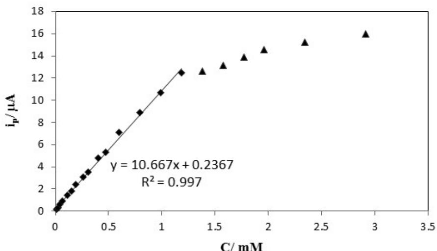
**Fig. 6.** Calibration plot for concentrations of INH from differential pulse voltammograms.
