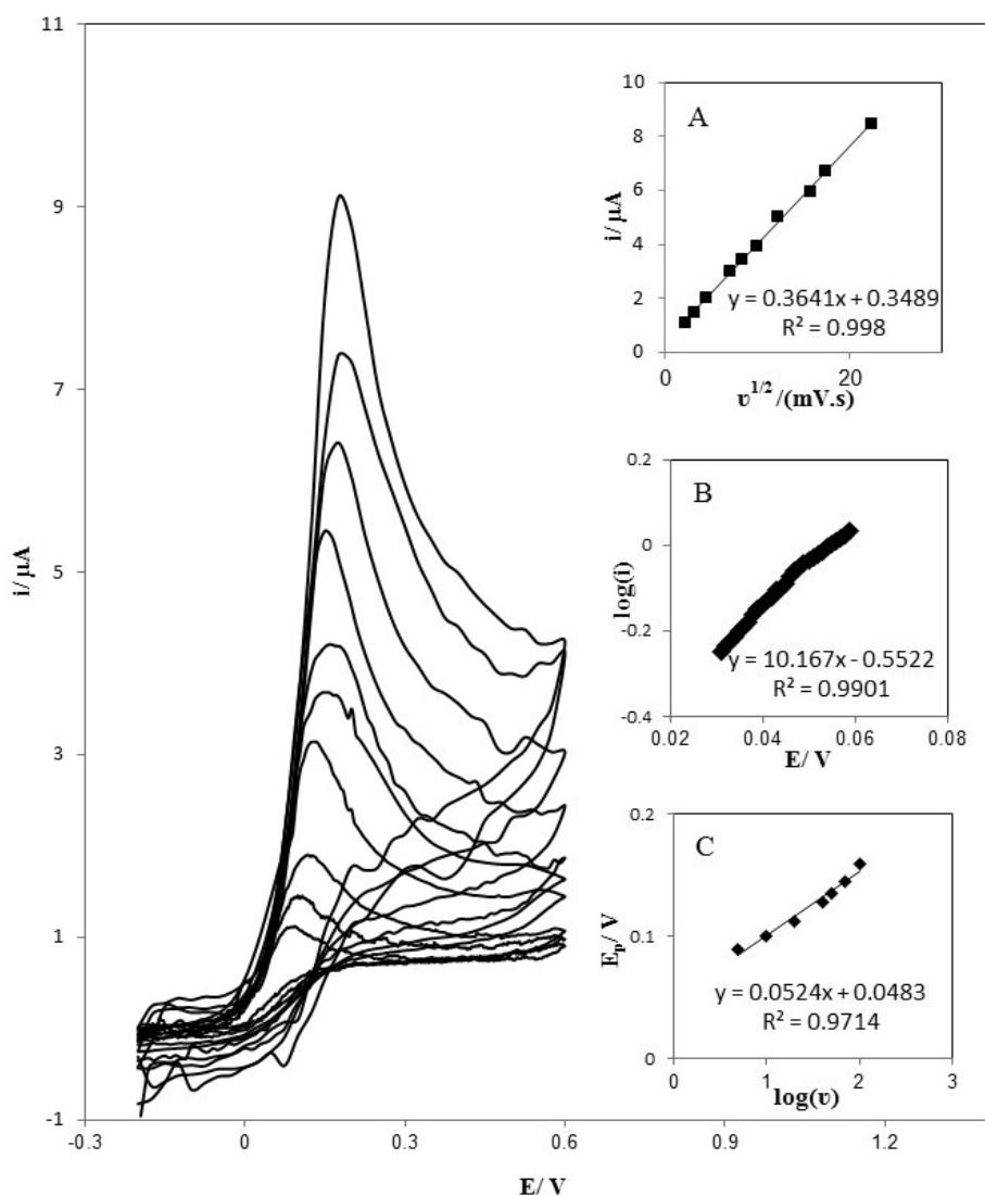
**Fig. 3.** Dependence of the cyclic voltammetric response at a poly(EBT) modified glassy carbon electrode in 0.1 M ammonia buffer (pH 9) containing 1 mM INH. Scan rate: 5, 10, 20, 50, 70, 100, 150, 250, 300 and 500  $\text{mV s}^{-1}$ , respectively. Inset A: Dependence of the peak current with square root. Inset B: Tafel plot derived from the rising part of voltammogram recorded at a scan rate 10  $\text{mV s}^{-1}$ . Inset C: plot of  $E_p$  vs.  $\log v$ .
