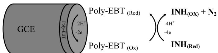
*Scheme 2.* Mechanism of INH oxidation on the poly-EBT GC modified electrode
