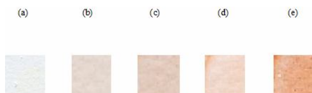
Fig. 4. Surfaces of TLC with (a) 0.0 \mu l, (b) 3.0 \mu l, (c) 6.0 \mu l (d) 9.0 \mu l and (e) 12 \mu l of QDs.
