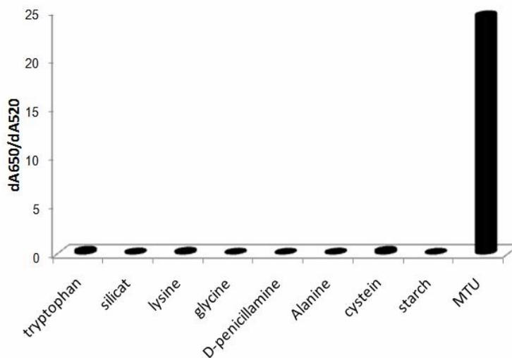
**Fig. 5.** The  $dA_{650\text{ nm}}/dA_{520\text{ nm}}$  value of solution in the presence of 0.1 mM tryptophan; silicat; lysine, glycine; D-penicillamine; alanine; cystein; starch and 2 $\mu\text{M}$  MTU.
