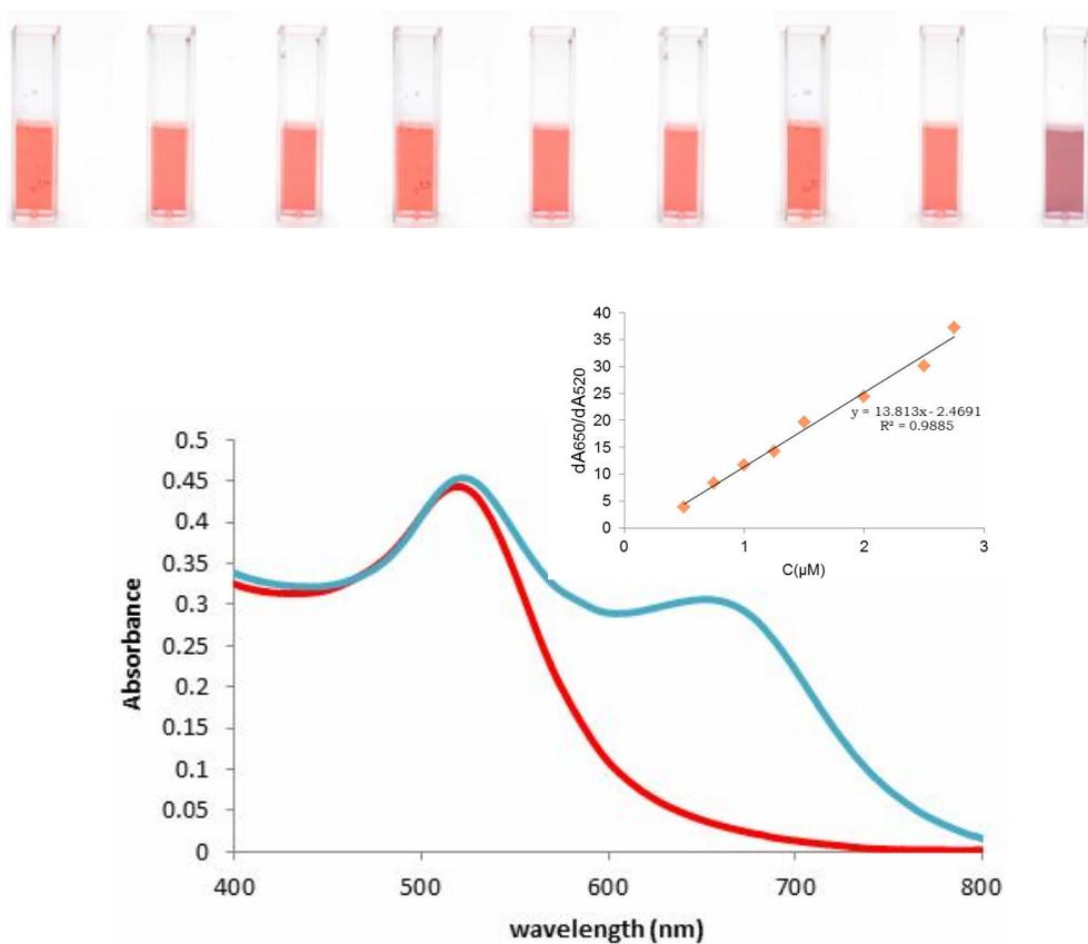
**Fig. 4.** A typical absorption spectra and digital photos of Au-NPs upon adding certain quantity of MTU (the insets are corresponding calibration curve in the range of 0.5-2.75  $\mu\text{M}$ ).
