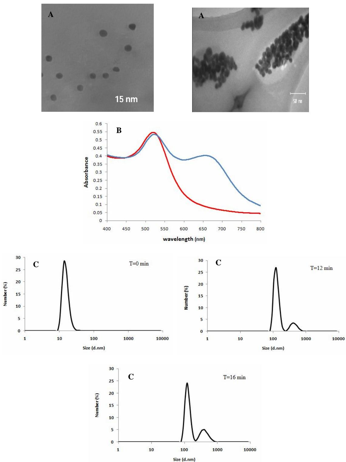
**Fig. 1.** (A) Typical TEM images; (B) corresponding UV-Vis absorption spectra; and (C) size distribution of the Au NPs before and after the addition of certain quantity of MTU.
