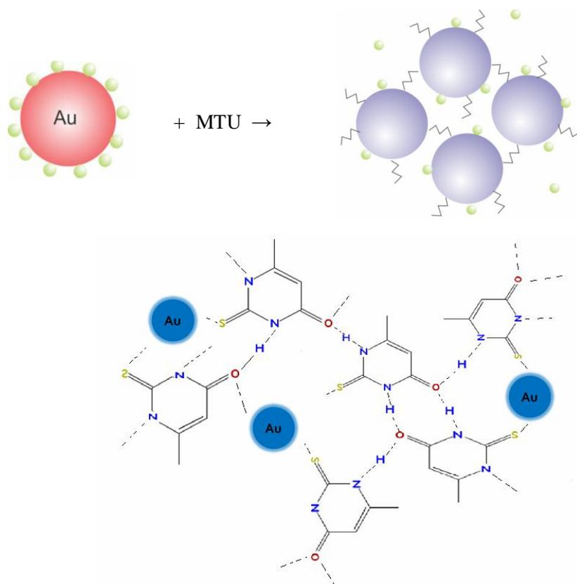
*Scheme 2.* Schematic illustration of the aggregation mechanism for MTU
