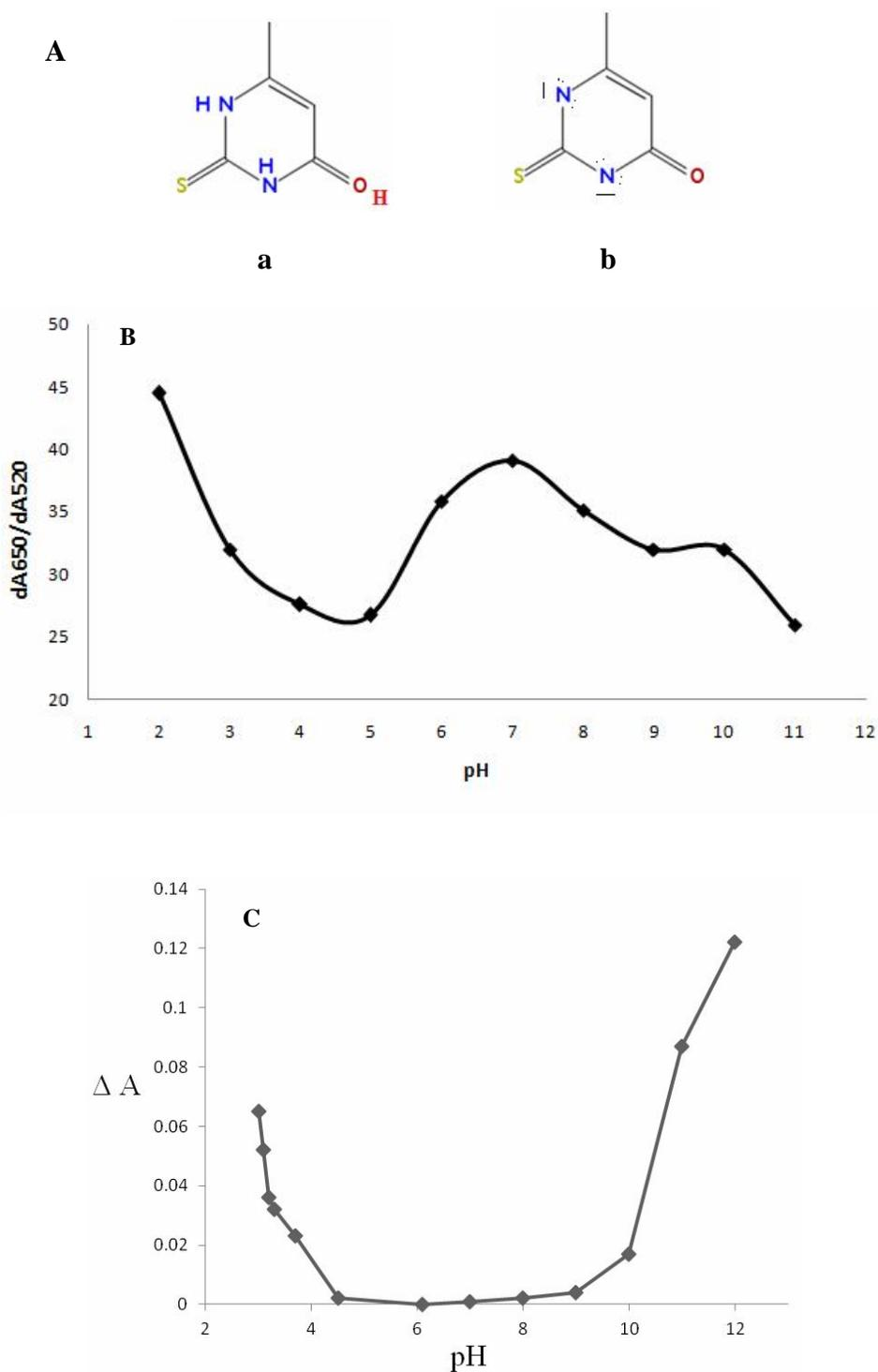
**Fig. 2.** (A) Schematic illustration of the structures of MTU in a) acidic and b) alkaline solution; (B) The effect of the pH of analyte solution on the self-aggregation of Au-NPs in the presence of analyte; and (C) effect of pH on the self-aggregation of Au-NPs in the absence of analytes.
