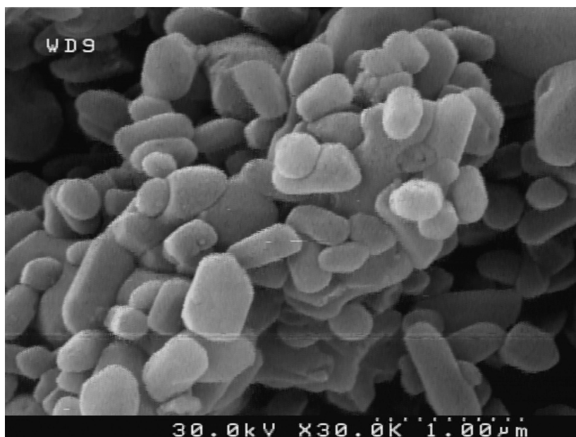
Fig. 3. A) X-ray diffraction pattern of TMU-24. B) SEM images of TMU-24.
